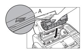
8 Insert the toner cartridge so that the guide (A) on the left side of the toner cartridge fits into the groove inside the machine and slide it down parallel to the guide.
